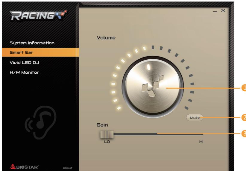
1. **Volume Control Knob:** The volume can be finely adjusted by turning the knob either clockwise or anti-clockwise to increase or decrease system volume accordingly.
