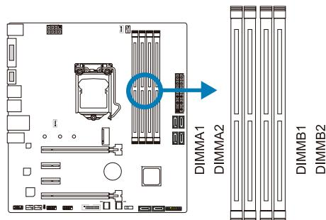
Step 1: Unlock a DIMM slot by pressing the retaining clips outward. Align a DIMM on the slot such that the notch on the DIMM matches the break on the slot.
