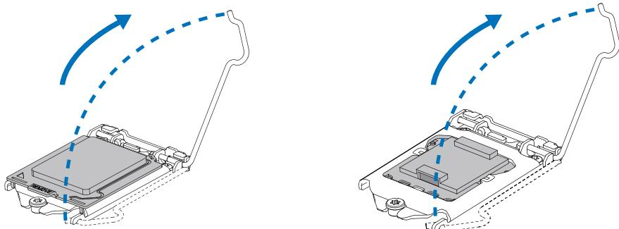
Step 3: Remove the Pin Cap.
