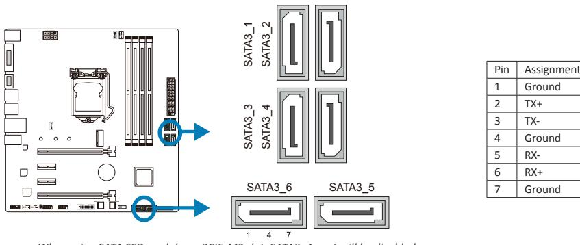
» When using SATA SSD module on PCIE-M2 slot, SATA3\_1 port will be disabled.
