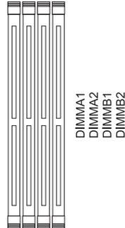
Step 1: Unlock a DIMM slot by pressing the retaining clips outward. Align a DIMM on the slot such that the notch on the DIMM matches the break on the slot.
