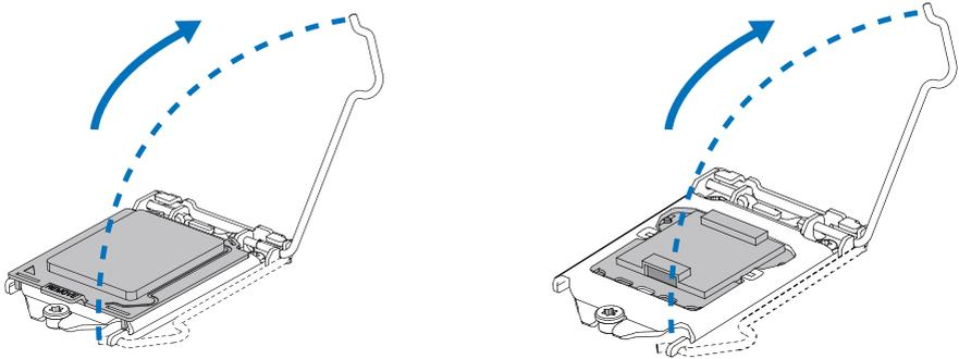
Step 3: Remove the Pin Cap.
