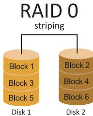
In a RAID 0 system data are split up in blocks that get written across all the drives in the array. By using multiple disks (at least 2) at the same time, this offers superior I/O performance. This performance can be enhanced further by using multiple controllers, ideally one controller per disk.
