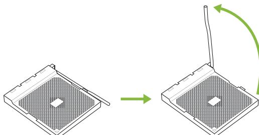
Step 3: Look for the white triangle on socket, and the gold triangle on CPU should point towards this white triangle. The CPU will fit only in the correct orientation.
