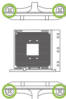
Step 2: Place the heatsink and fan assembly on top of the installed CPU and make sure that the fan cable is closest to the CPU fan connector. Please refer diagram to the following screw into the screw hole in the order shown.
