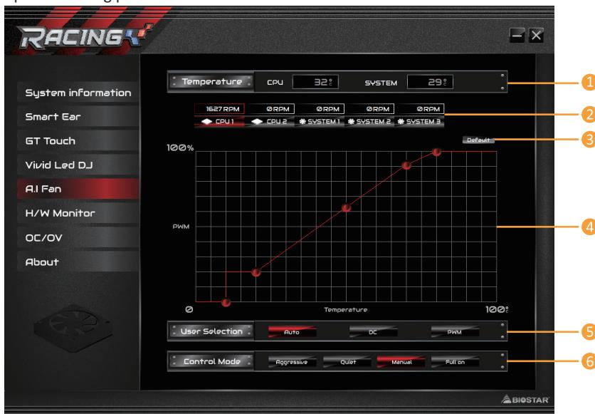
1. **Temperature:** Shows the current CPU and system temperature.
