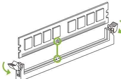
Step 2: Insert the DIMM vertically and firmly into the slot until the retaining clips snap back in place and the DIMM is properly seated.
