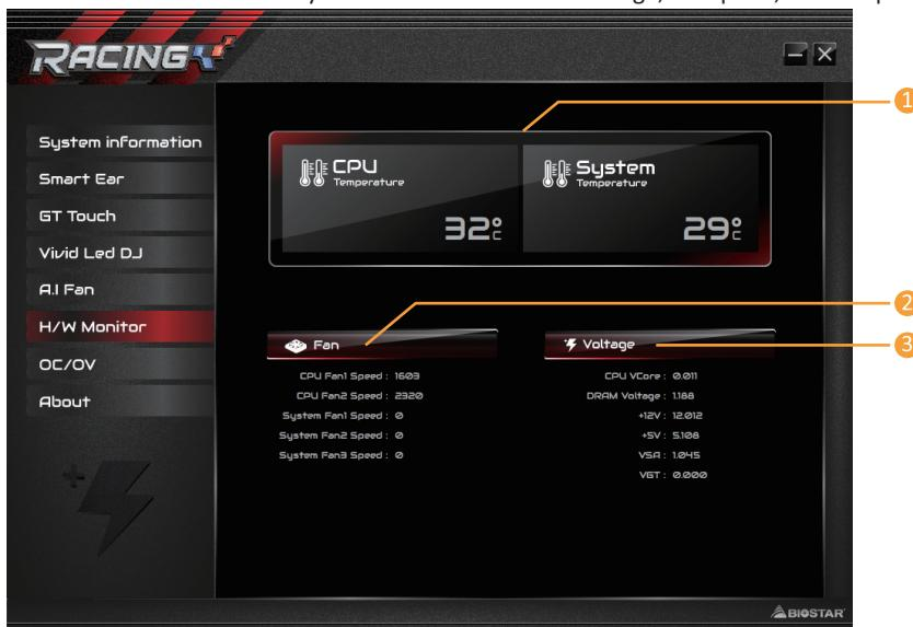
1. **CPU Temperature/System Temperature:** Shows the current CPU and system temperature.
