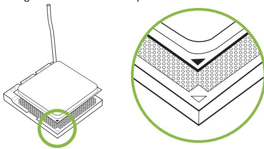
Step 4: Hold the CPU down firmly, and then close the lever to locked the position
