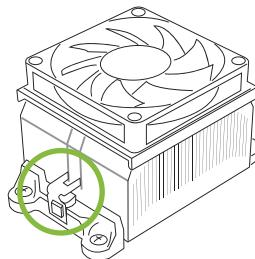
Step 2: On the other side, push the retention clip straight down to lock into the plastic lug on the retention frame, and then press down the locker until it stops.
