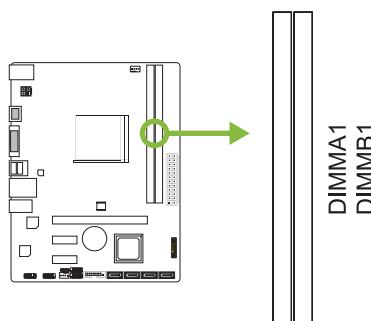
Step 1: Unlock a DIMM slot by pressing the retaining clips outward. Align a DIMM on the slot such that the notch on the DIMM matches the break on the slot.
