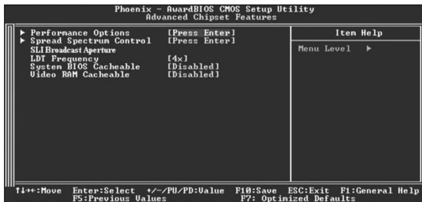
■ Figure 4. Advanced Chipset Setup
