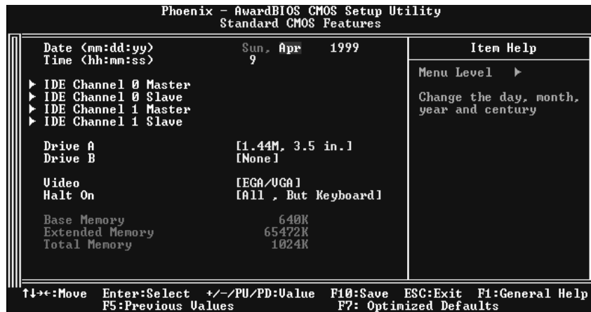
■ Figure 2. Standard CMOS Setup
