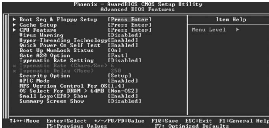
■ Figure 3. Advanced BIOS Setup
