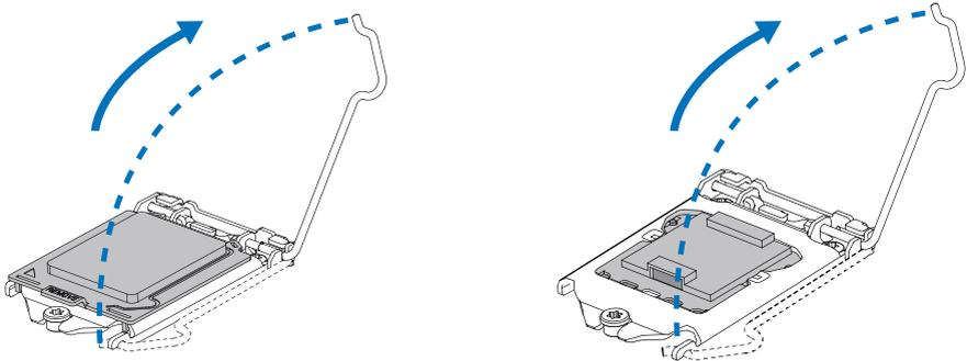
Step 3: Remove the Pin Cap.
