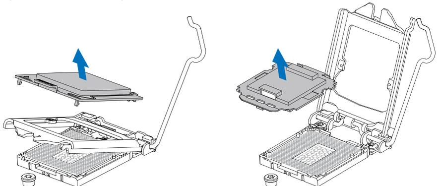
Step 4: Hold processor with your thumb and index fingers, oriented as shown. Align the notches with the socket. Lower the processor straight down without tilting or sliding the processor in the socket.
