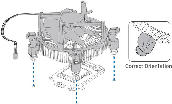
Step 2: Press down two fasteners at one time in a diagonal sequence to secure the CPU fan assembly in place. As each fastener locks into position a click should be heard.
