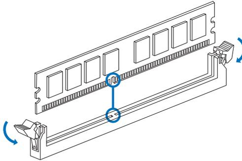
Step 2: Insert the DIMM vertically and firmly into the slot until the retaining clips snap back in place and the DIMM is properly seated.
